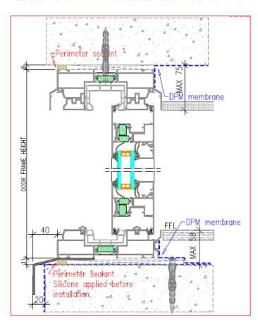
When a "flush threshold" has been specified then the height of the frame is given from the top of the frame down to the FFL. The threshold is allowed to them be let into the floor allowing the external level to match the internal level. The upstand should be build 58mm below FFL
