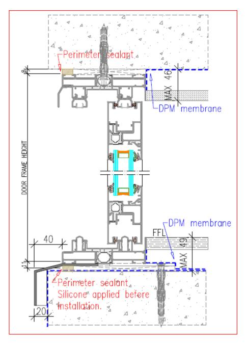
When a "flush threshold" has been specified then the height of the frame is given from the top of the frame down to the FFL. The threshold is allowed to them be let into the floor allowing the external level to match the internal level. The upstand should be build 49mm below FFL
